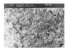
**Figure 12** Scanning electron micrograph of impactfractured specimen of MMA-*g*-EPDM–PVC (4% grafting).
